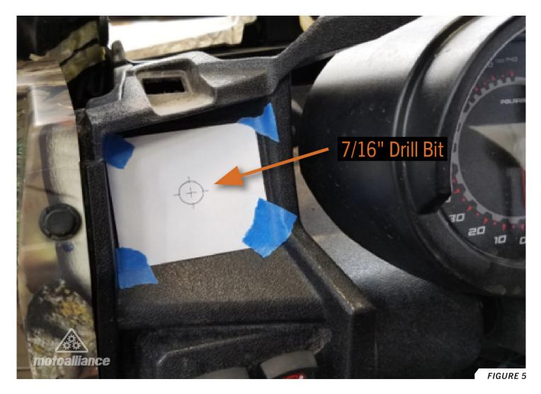
10. Mark the center of each hole and drill using the corresponding bit or hole saws. Remove any plastic burrs from the holes.
